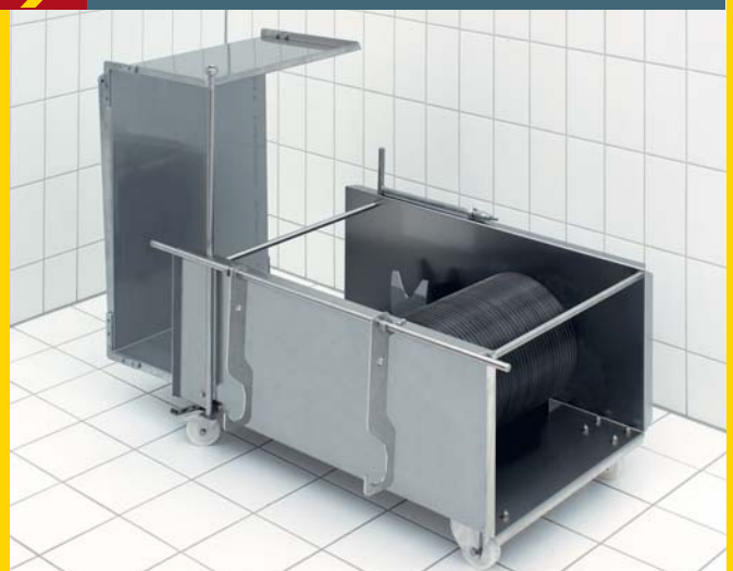
Cleaning wagon for 2 blades shafts (cover open, lift-out-device hung in)
