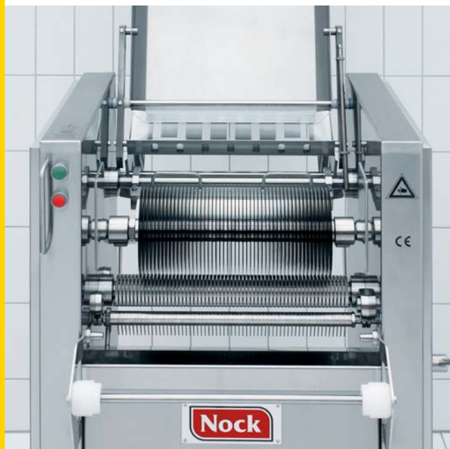
Cortex CB 495/5K SLICER after removing the conveyor belts
