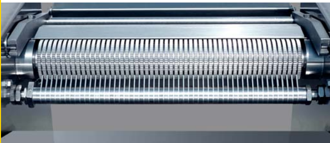
Transport roller with medium or coarse toothing and scrapper comb in the NOCK models CBF and CF
