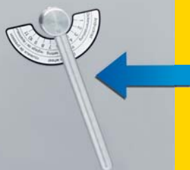
Operating lever for adjusting the height of the pressure roller
