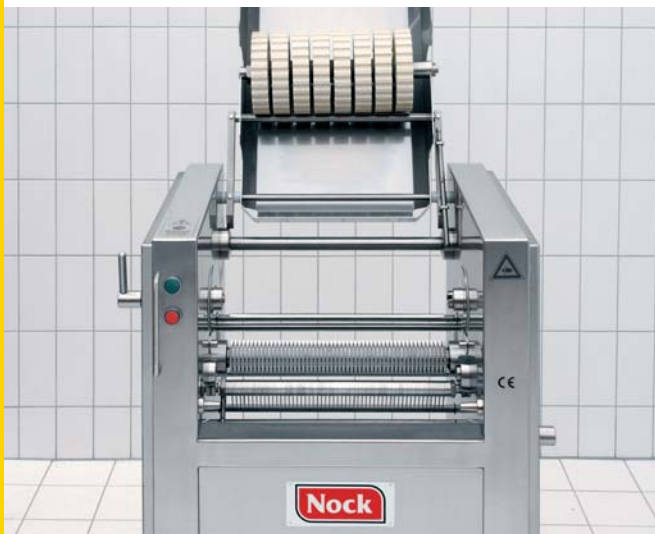
Quick and easy to clean: NOCK derinder after removing conveyor belts, pressure roller and blade holder. Scrapper comb tilted back.
